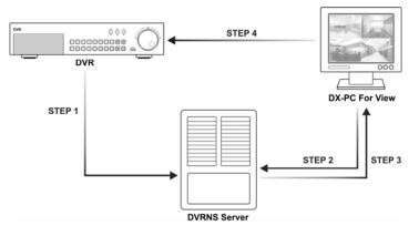
STEP 1 (DVR  $\rightarrow$  DVRNS Server): Register the unit name and IP address of the DVR during the DVRNS setup on the Remote DVR. This unit name and IP address will be registered on the DVRNS server directly.
